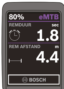
Figure 8 - Braking behaviour information screen on the Kiox display.
