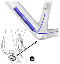
After fitting the battery int the frame, close the hole below the bottom bracket using Battery Rubber cap (N.22)
