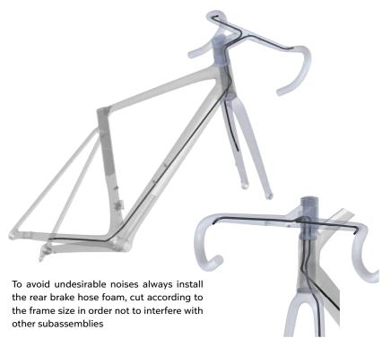
To ease the procedure it is recommended to route the brake hoses before installing the headset and the Di2 battery.
