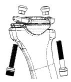
**NOTE:** seatpost 0-offset must be fixed with the 2 bolts from the bottom, featured with the dedicated spherical washers (N. 4.5)
