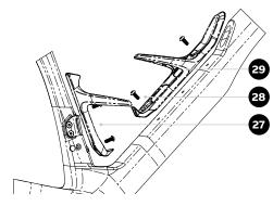
Fix the DT and ST custom bottle cages (N.29 and N.27) with the dedicated screws (N.28). In case of Di2 setup, follow Step 1 before. Colnago Y1Rs is compatible with conventional bottle cages; however, clearance and bottle handling depend also and the adopted brand and model and must be checked by the user.
