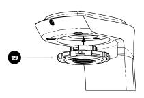
**Step 3:** Fit the preload gear (N.19) into its seat in the lower face of fork top plate.
