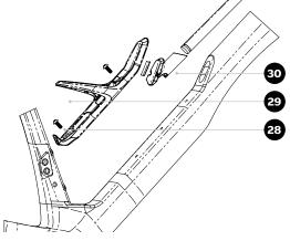
In case of Shimano Di2 groupsets, insert the battery into the battery support (N.30) and fix with a zip-thight or similar. Then, fix the battery support to the DT Bottle cage (N.29) with the provides sticky tape. Connect Di2 cables already routed in the frame and insert the battery in the hole on the downtube and screw as shown in the picture.
