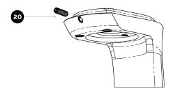
**Step 1:** Before to assemble frame and fork, remove the M5X16 headless screw (N.20), if already fitted in the fork top plate.
