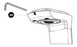
**Step 12:** Fix the M5x16 headless screw (N.20) removed in Step 1 in the rear side of fork top plate till its point touches the preload gear, in order to prevent its unscrewing.
