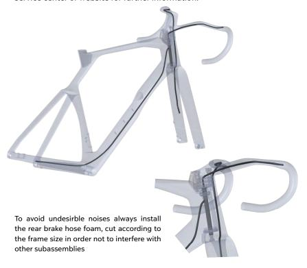
Before to route the brake hoses it is recommendable to install the headset and fork following the Steps 1 and 2 in the dediceted section. Once installed and routed the rear brake hose in the dowtube, with a dedicated wiring tool with magnet in the end, pull the it through the preload bolt hole as shown in the pictures below.
