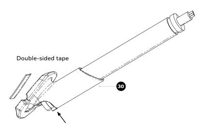
Insert the Di2 battery in the Di2 Battery Support (N.30). Use a thin zip tight to secure the battery using the rear battery groove, as shown by the red arrow. Apply double-sided tape as shown in the picture to fix the battery support to the bottlecage, once both of them are installed.
