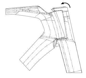
**Step 4:** Keeping the preload gear in its seat (Step 3) and all the frame head tube components in theirs (Step 2), insert the fork in the frame head tube as shown in the picture, starting from the lower part and applying a rotation around the lower bearing.
