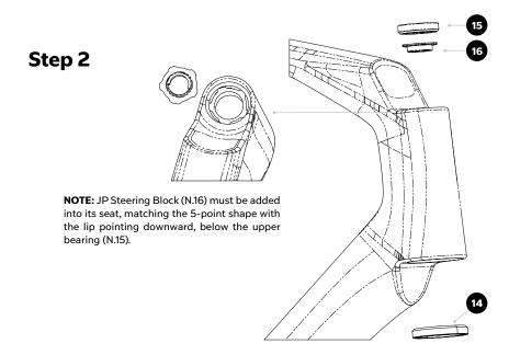
**Step 2:** Apply a thin layer of dedicated bearing grease in bearing seats and put in their seats in the Head Tube the JP steering block (N.16), upper (N.15) and lower (N.14) bearings, in this order, as shown in the picture.
