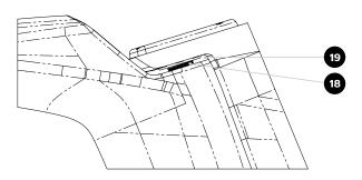
**Step 9:** Once counterclock rotation is not possible anymore, the head of preload bolt (N.18)must be fully into the fork top plate and the preload gear (N.19) should be raised with respect to the frame from lateral view.
