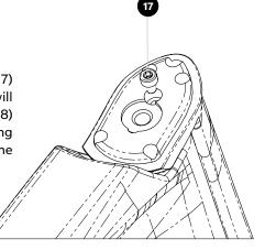
**Step 8:** Firmly holding the preload bolt (N.18) head and screw from the side the preload gear counterclock wise with the dedicated tool (N.32). The head of the preload bolt (N.18) will go down till it fits in its seat. The preload head matching the shape of the M4x8 screw (N.17) will prevent unwanted rotations of the bolt.
