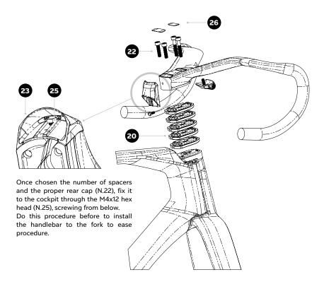
After adding the desired number spacers (N.20) up to a maximum of 5, fix the handlebar (previously equipped with the custom rear cap according to the spacer height). Using 4 M6 screws whose lengths depend on the number of spacers (check 'Screws and cap choice' section), to fix the handlebar applying a torque of 6 Nm in each screw. Finally cover the screaw head with the dedicated caps (N.26)
